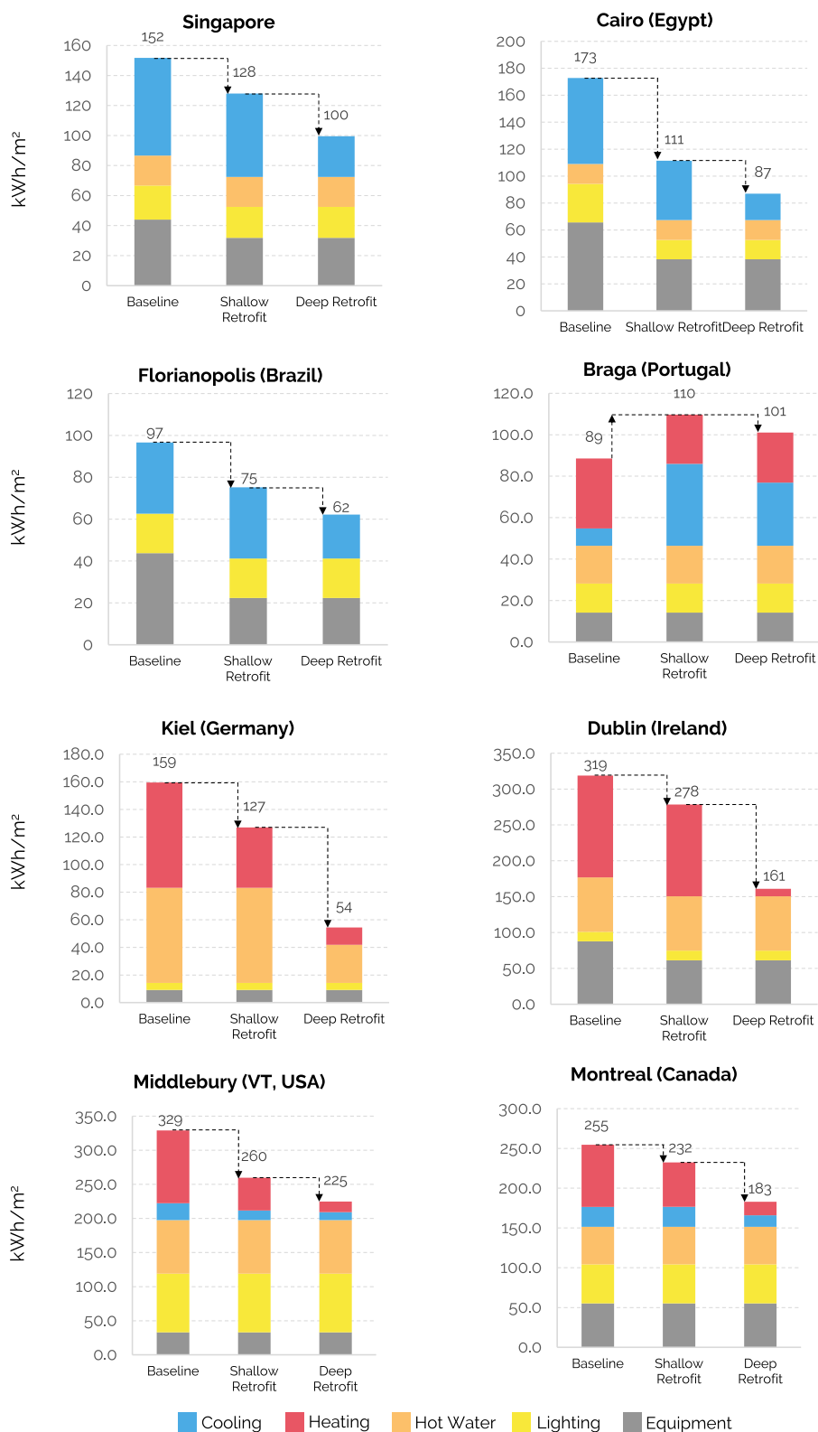
Fig. 2 | Energy Use Intensities (EUI) for the baseline and retrofit scenarios for eight cities. A baseline and two additional scenarios are defined for each city, with the colors representing energy use intensities for various end uses. Shallow retrofits naturally lead to smaller reductions in EUI, while deeper retrofits require
