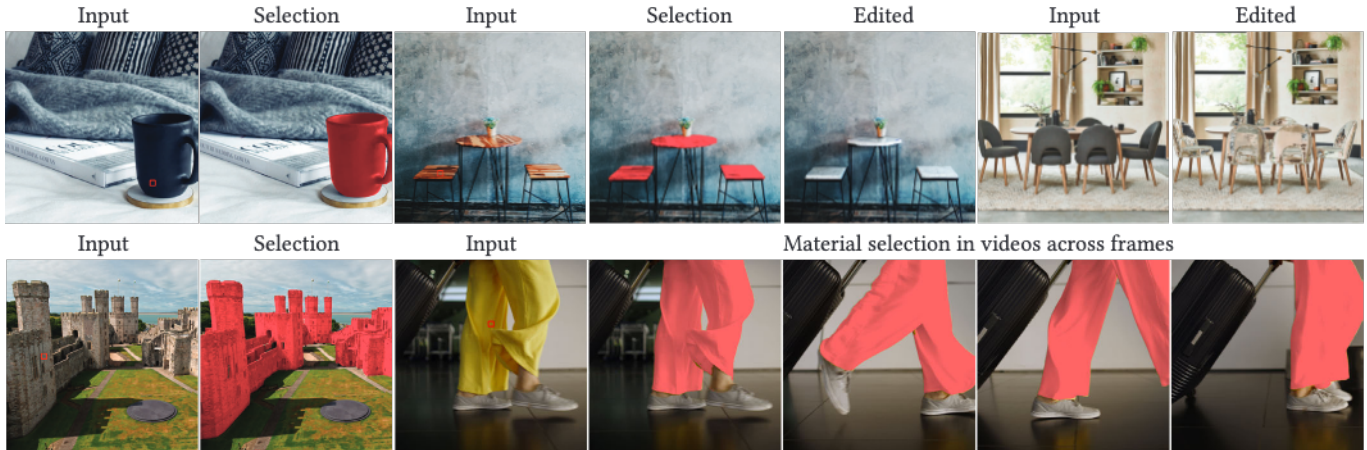
Fig. 1. Given an input image and a pixel selection (marked with a red square), our method automatically selects all the pixels that have the same material as the query. Our algorithm can identify materials shared by different objects (table and stools), and is robust to shading variations (castle example). Material-based selection enables downstream applications, such as material editing or replacement (top right). Our approach can be extended to select materials across multiple images, enabling material selection in videos (bottom right) without requiring any optical flow propagation.
