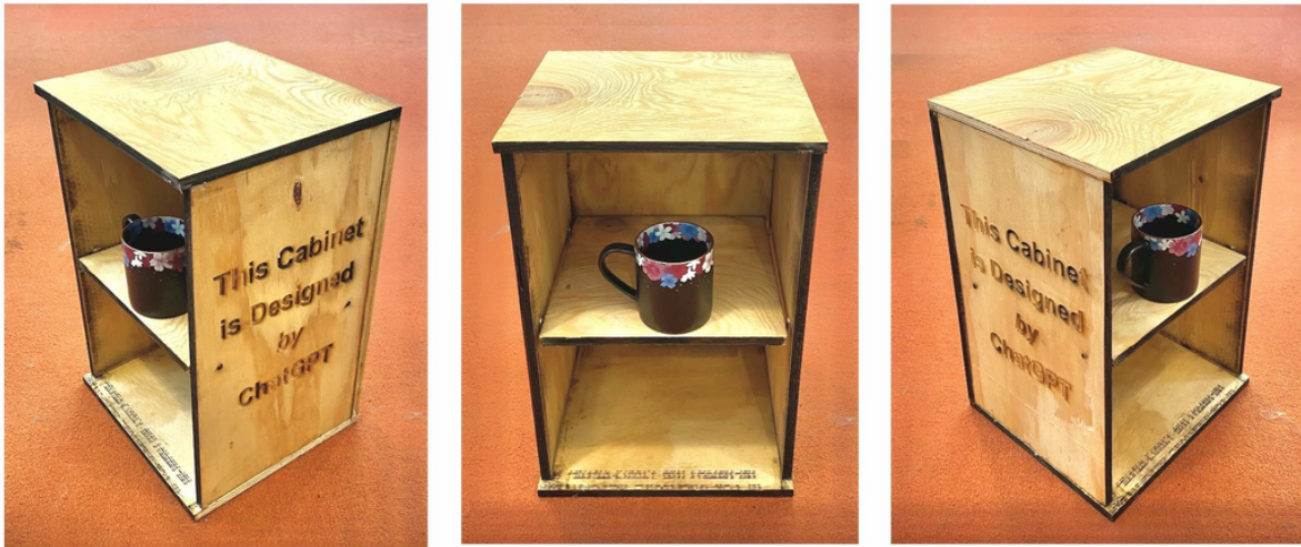
Fig. 70. The Manufactured Cabinet. Real-world cabinet manufactured from different view angles, showcasing its scale with a mug as a reference.
