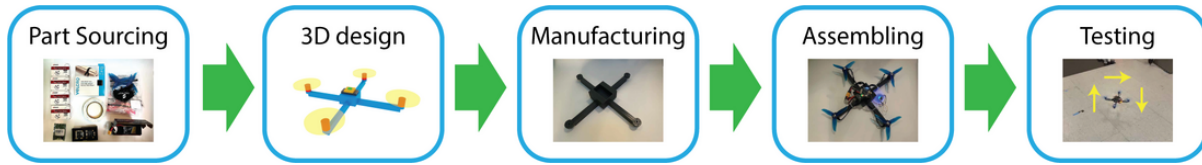
Fig. 72. The Quadcopter Design Process using GPT-4. The process involves sourcing parts, creating a 3D design, manufacturing, assembling and testing the quadcopter. We successfully manufactured a working quadcopter.
