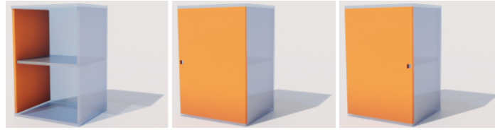
Fig. 17. Adding a door to an existing cabinet. We provide GPT-4 with the initial cabinet design from Section 4.1.4 (semi-transparent blue), then ask it to add a door (orange) with a handle on the right-hand side. Despite beginning from a largely-complete model, GPT-4 still has difficulty placing the door and handle correctly.
