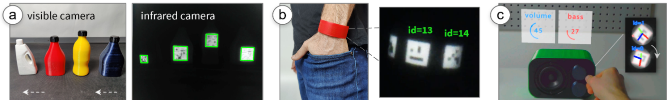
Figure 1: BrightMarkers are embedded into objects using a NIR-fluorescent filament. (a) When viewed with a NIR camera with the matching filter, the markers appear with high contrast, which allows them to be tracked even when the objects are in motion, e.g., on a conveyor belt. (b) BrightMarker can be used to fabricate custom wearables for tracking, or (c) for transforming physical controls into precise input methods in mixed reality environments.
