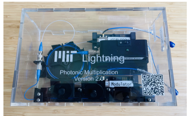
Figure 26: LIGHTNING’s photonic computing developer kit.
