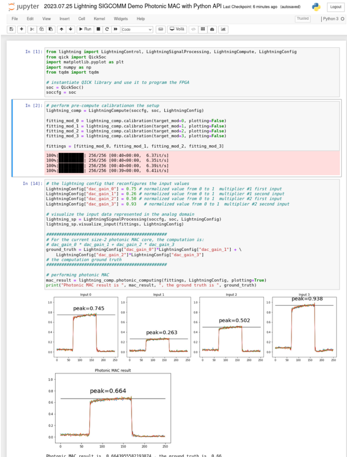
Figure 27: Benchmarking photonic vector dot product on LIGHTNING’s prototype with our Python API.
