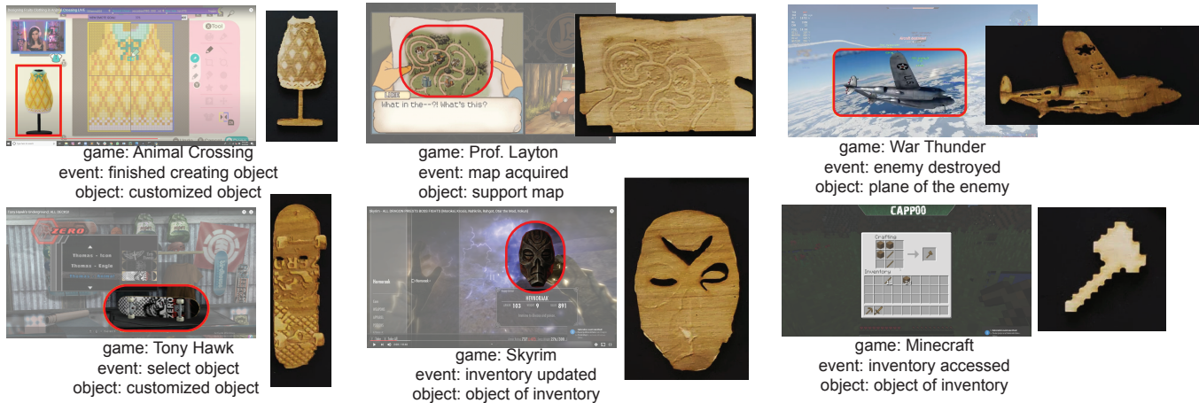
Figure 3: Examples of gameplay moments from the study that were integrated with fabrication events, and their respective fabrication objects laser cut from the auto-generated fabrication files from the study. (a) In the game Animal Crossing , when the player finishes the custom design of the dress, they can fabricate their final design. (b) In the game Prof. Layton , when the player acquire a map, they can fabricate its physical version. (c) In the game War Thunder , when the player destroys their enemy's aircraft, they can fabricate the fallen aircraft. (d) In the game Tony Hawk , when the player chooses their custom skateboard, they can fabricate the skateboard design. (e) In the game Skyrim , when the player's inventory updates with a rare mask, they can fabricate the custom mask. (f) In the game Minecraft , when the player's inventory of tool is accessed, they can fabricate the tool.
