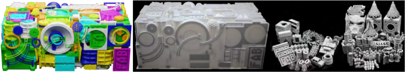
Fig. 9. Left: A packing with a density 34.25\% produced by our algorithm. Middle: The packed tray printed with an inkjet printer. Right: The disassembled parts.
