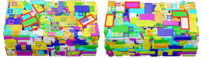
Fig. 18. Left: PIECES packed by evenly searching 30^\circ over Euler angles. It produces a sub-optimal result with a density of 44.91%. Notice misaligned parts as highlighted. Right: The same dataset packed by only searching 90^\circ . This results in a better density of 50.81% where parts are axis aligned.
