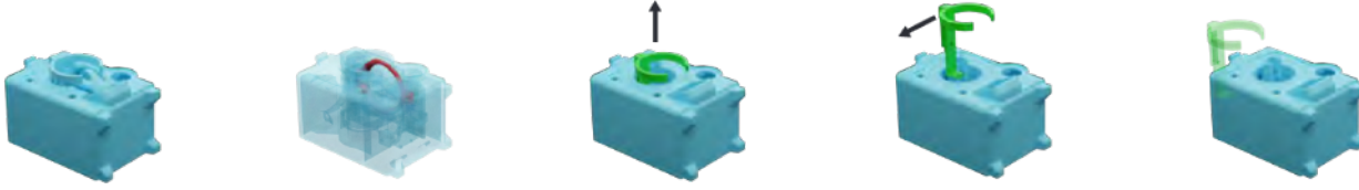
Fig. 5. Flood-fill disassembly. From left to right: The algorithm checks if each object can be physically disassembled. An object may be removed if no other objects can be disassembled. For example, the ring object marked with red is removed in the second figure. Once the interlocking is resolved, the algorithm iterates over the remaining objects, and removes them following a physically valid path.
