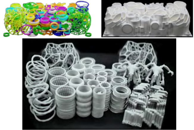
Fig. 21. Top left: The same set of objects in Fig. 20 are packed with our algorithm with no interlocking. Top right: The printed tray containing the set of objects on the left. Bottom: The disassembled printed objects.
