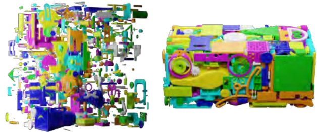
Fig. 23. Left: The packing result of MIXTURES with pack3d, where it fails to converge with a packing density of 3.47\% after 1200s. Right: Our algorithm achieves a packing density of 34.71\% in only 67.99s.
