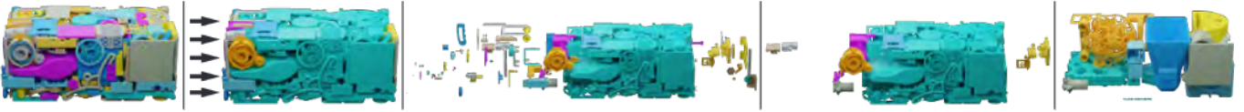
Fig. 6. Ray-casting disassembly. From left to right: Starting with a packed tray, we cast rays along the x direction shown with the black arrow. A DBG is obtained, where SCCs are rendered with the same color. Then, every SCCs with only one object are disassembled from the packing, as shown in the third and fourth figure. This broad-phase disassembly is repeated several times along different directions. The remaining SCCs are shown in the fifth figure.
