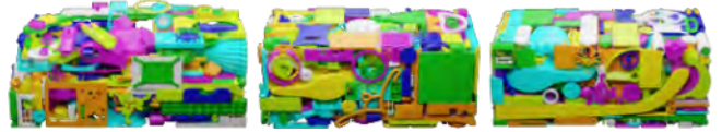
Fig. 19. Left: Placing parts in random order produces sub-optimal result with a density of 29.9%. Middle: Placing parts from largest to smallest produces a better packing density of 34.71% with the same computational cost. Right: Beam search results in a packing density of 35.06%, but spends 4 \times more time.
