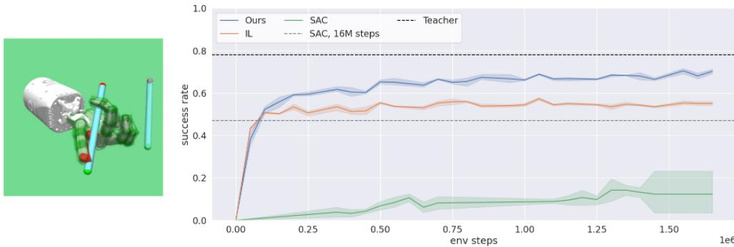
Figure 2: Success rate of a pen reorientation task by Shadow Hand robot, using tactile sensing only. While vanilla reinforcement learning takes a long time to converge, and imitation learning methods can suffer from Imitation Gap, our algorithm is able to solve the task with reasonable sample efficiency.
